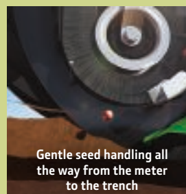
BrushBelt system eliminates seed bounce
