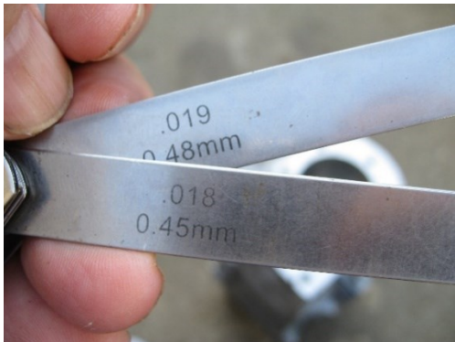
Figure 7. These two feeler gauges together are used to check middle compression ring end gap. Use the combined feeler gauges to calculate the ring end gap.
