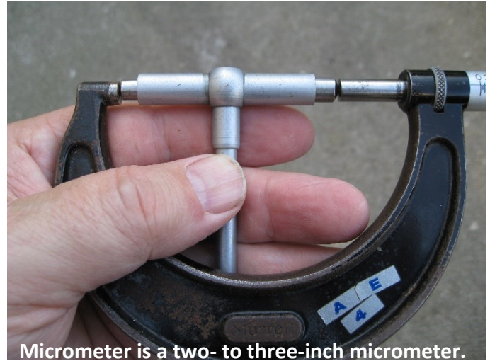
Figure 2. Illustration of using an English micrometer to take a reading from the telescoping gauge.
