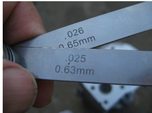
Figure 8. These two feeler gauges together are used to check oil ring end gap. Use the combined feeler gauges to calculate the ring end gap.
