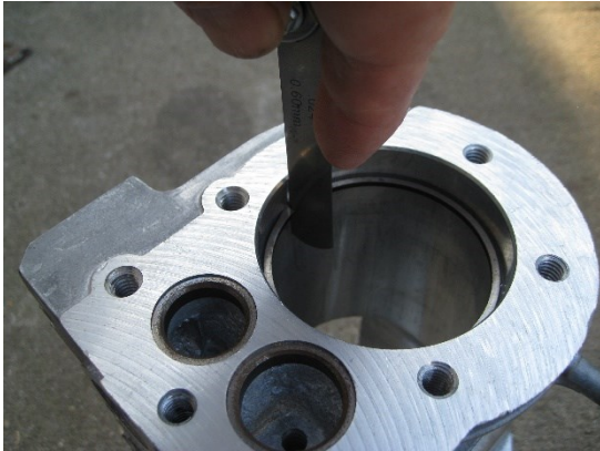
Figure 5. Illustration of using a feeler gauge to check end gap of rings.
