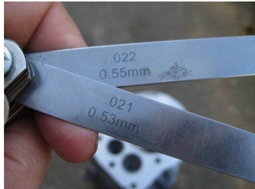
Figure 6. These two feeler gauges together are used to check top compression ring end gap. Use the combined feeler gauges to calculate the ring end gap.
