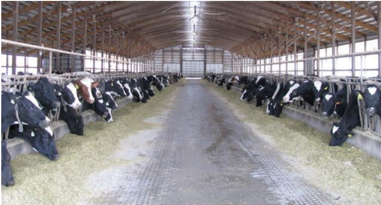
Figure 1. Free stall barn at FFA Family Dairy. The barn is a curtain-sided free stall barn with an open ridge, a central feed alley, and fans that are set to automatically turn on at 78 degrees F.
