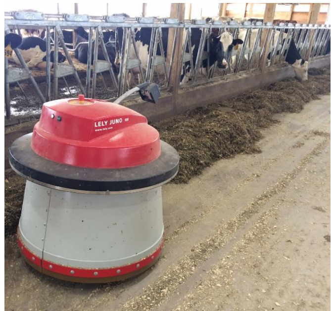
Figure 1. Automatic feed pusher that pushes up feed every hour for 22 hrs per day.
