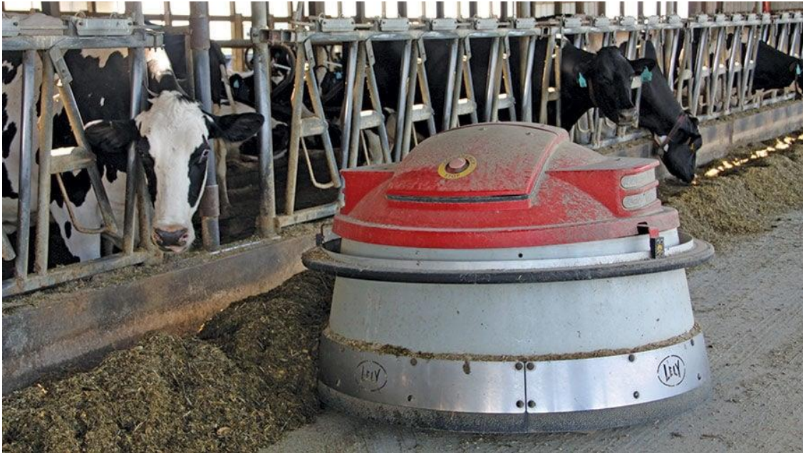
Figure 3. One example of a rotating feed pusher. (Photo credit: https://agupdate.com )
