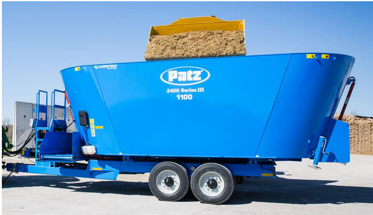
Figure 1a. The double screw TMR mixer used for feeding the cows at FFA Dairy.
