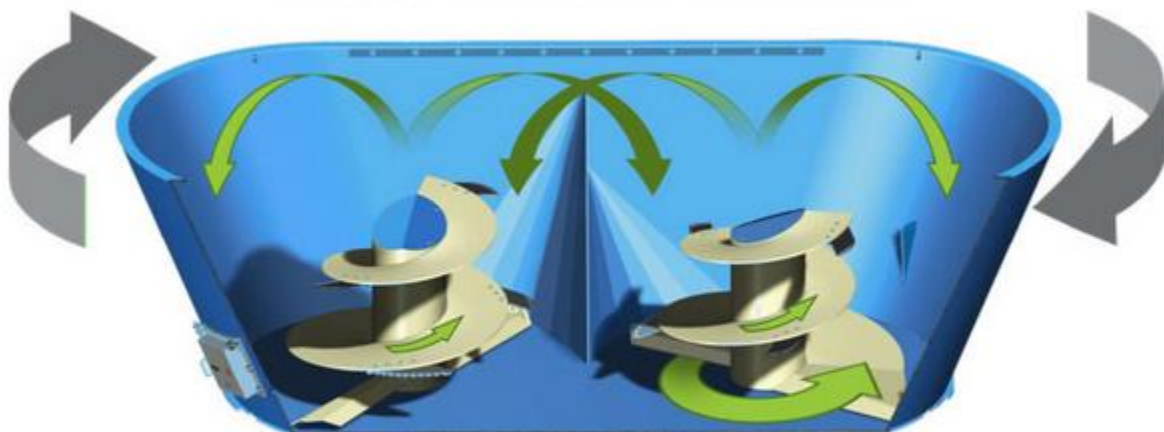
Figure 1b. Diagram of how the double-screw TMR mixer works to mix the feed. (Photo credit: https://www.agcentral.coop/dairy-services/patz )
