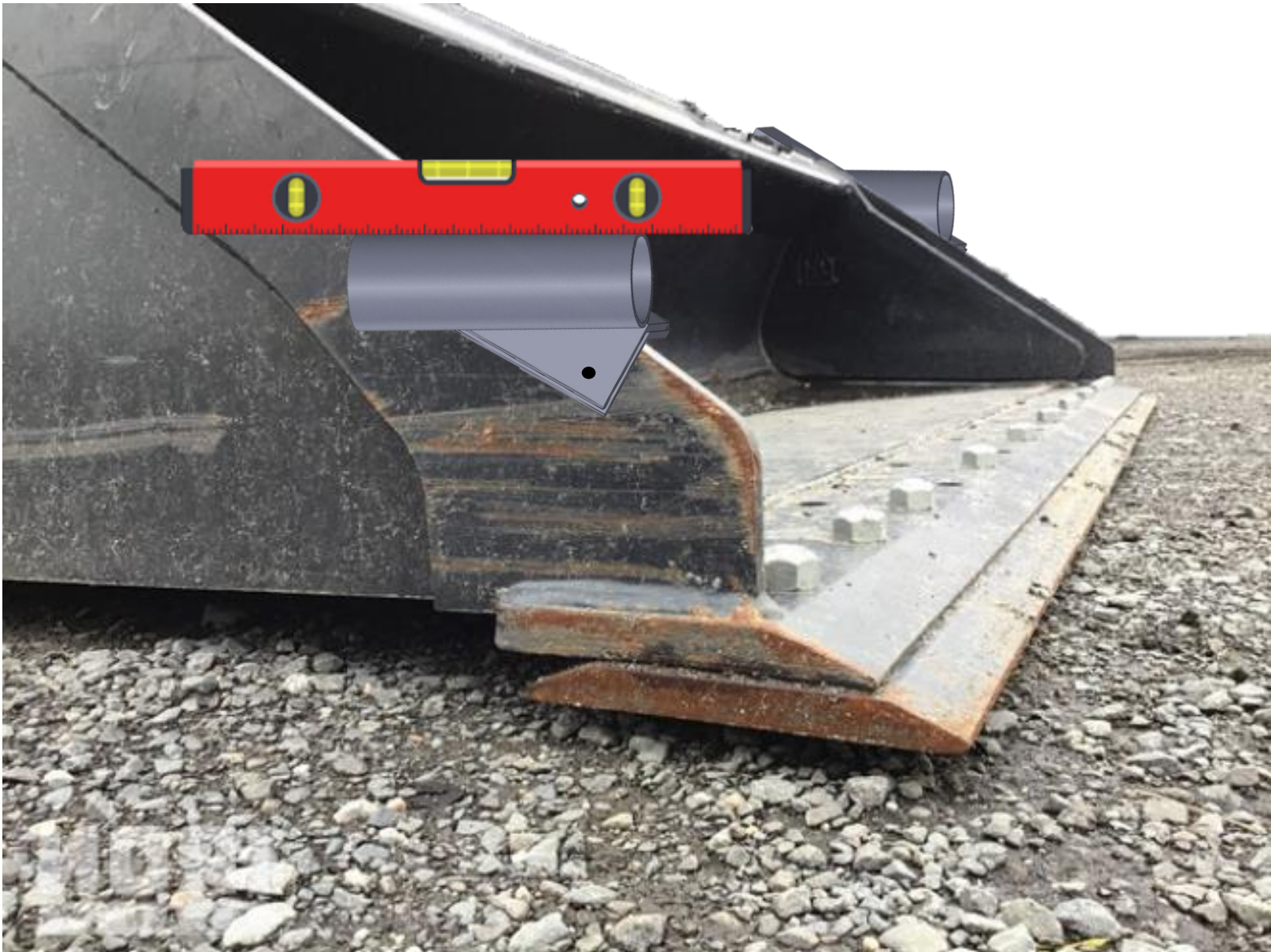
Figure 2. Illustration of leveling the Spear Bracket.
