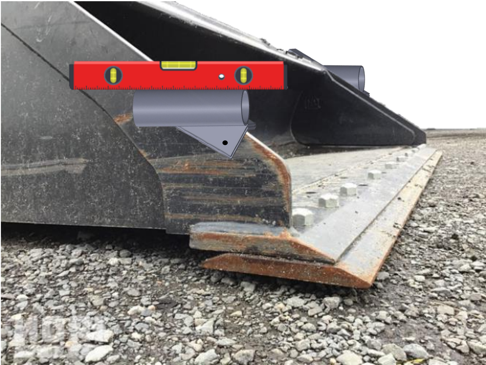
Figure 2. Illustration of leveling the Spear Bracket.
