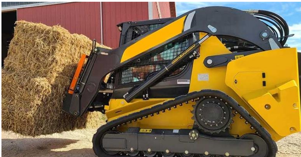
Figure 4. Example of a skid steer with spears to move large bales.
