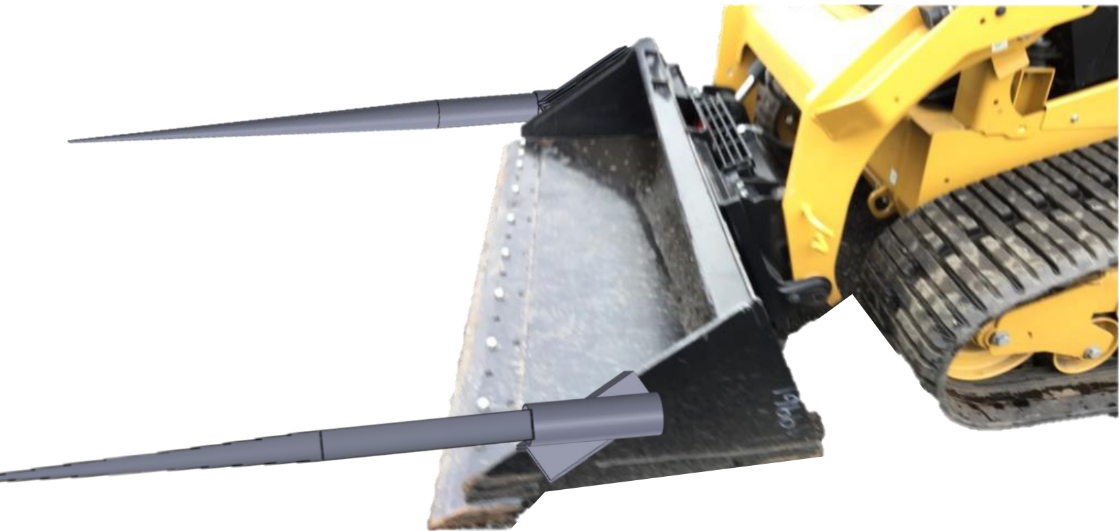
Figure 1. Illustration of bale spears and bracket for Caterpillar Skid Steer.
